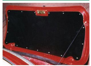
These black boot lid boards were fitted originally to MK.I cars in the 1960 period, but have proved very popular since as an accessory. The board is held in place with screws and cupwashers which are provided and will protect the paintwork and will probably give extra sound insulation.
